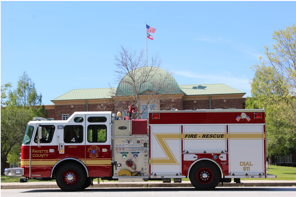
Photo 1: A 2018 Emergency One Fire Pumper, with a 450-HP Diesel Cummins engine, custom cab, and 1,000 gallon water take with a 1,500 GMP pump was ordered through the Purchasing Department during December 2017. Final steps are underway to place the truck in-service, with an expected date of June 2018. (similar make and model pictured)
