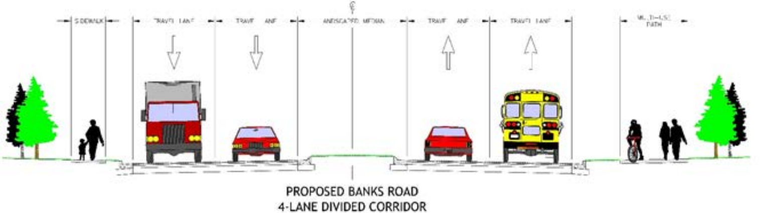
Graphic 5.2 - Banks Road Proposed Improvements Typical Section
