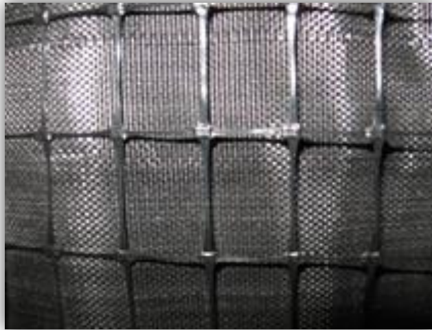
(Close up of C-Pop Silt fence)
