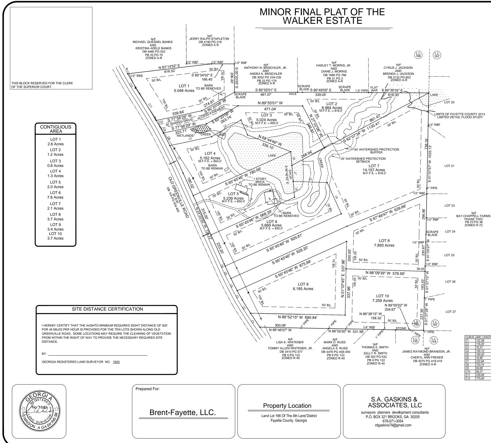
LEGEND **RBF=REBAR FOUND** RBS=REBAR SET CTP=CRIMP TOP PIPE L.L.=LAND LOT L.L.L.=LAND LOT LINE ₽ = PROPERTY LINE CO=CONSTRUCTION ENTRANCE EP= EDGE OF PAVEMENT P.O.B.=POINT OF BEGINNING **B/L=BUILDING SETBACK LINE** D.E.=DRAINAGE EASEMENT N/F=NOW OR FORMERLY F.W.P.D.=FIELD WORK PERFORMED DATE O/F=OUT OF FLOOD PLAIN DB=DEED BOOK PG=PAGE PB=PLAT BOOK ### =HOUSE NUMBER OTP= OPEN TOP PIPE
