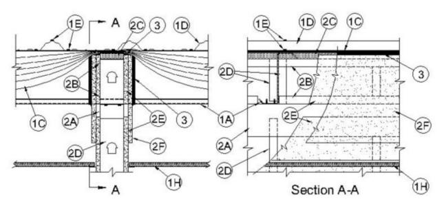
1. **Roof-Ceiling Assembly** — The fire rated roof-ceiling assembly shall be constructed of the materials and in the manner described in the individual P200 or P500 Series **Roof-Ceiling Designs** in the UL Fire Resistance Directory and shall include the following construction features:
