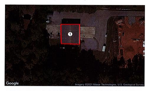
The current roof system is a Trapezoidal Metal Panel roof system estimated to be +/- 30 years of age in good condition. The repairs needed are as follows:
