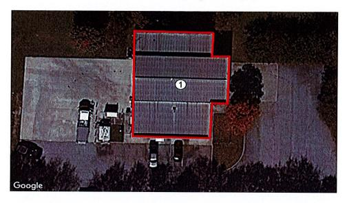
The current roof system is a Trapezoidal Metal Panel roof system estimated to be +/- 30 years of age in good condition. The repairs needed are as follows:
