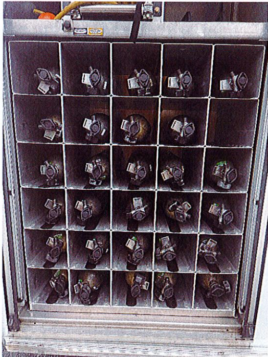
Grid/square bulk cylinder storage concept for compartment R4 but with additional slots for 48 total cylinders.
